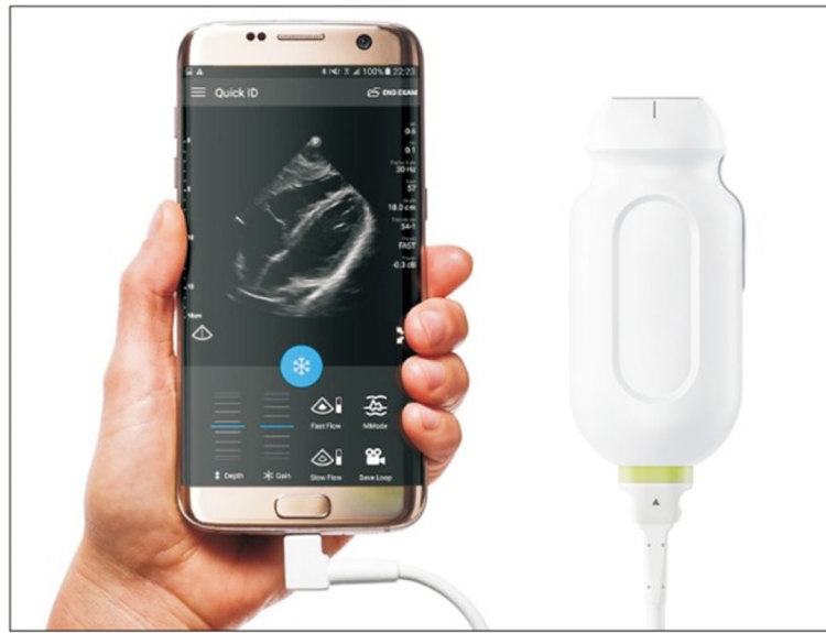
Fig. 1 Ultrasound machines for applications such as echocardiography, regional anesthesia or central line placement have now evolved to the point that they can be connected to a smartphone or tablet. Image from Michard F. Smartphones and e-tablets in perioperative medicine. Korean J Anesthesiol. 2017 Oct;70(5):493–499. doi: https://doi.org/10.4097/kjae.2017.70.5.493 . PubMed PMID: 29046768; PubMed Central PMCID: PMC5645581. Image used under the terms of the Creative Commons Attribution Non-Commercial License, which permits unrestricted non-commercial use, distribution, and reproduction in any medium, provided the original work is properly cited
