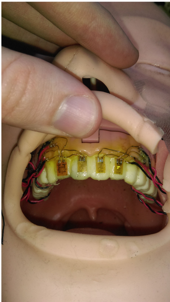
Fig. 1 Photograph of mannequin showing strain gauges attached to the upper incisors
