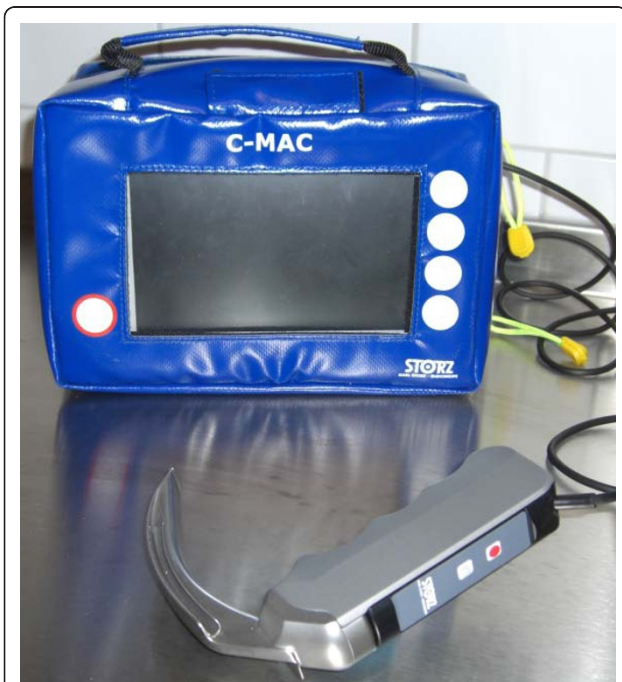
Figure 1 The portable C-MAC videolaryngoscope. The C-MAC videolaryngoscope, stored in the portable protective bag. Note the buttons for image recording on the monitor and the laryngoscope handle.
